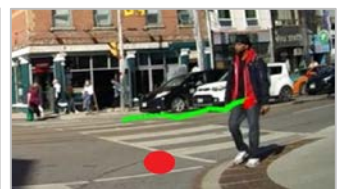
Active trigger with pedestrian prediction path inside RoI
