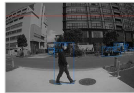
Captured image from front camera and Object detections
